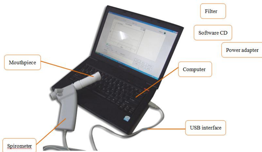
Structure of Handheld Spirometer
